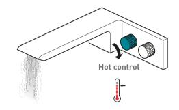
Turn the control clockwise to increase the flow of hot water
