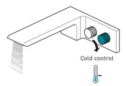
Turn the control clockwise to increase the flow of cold water
