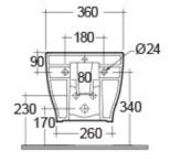
Dimensions: All dimensions in mm tolerance  $\pm 5\%$  for below 200mm and  $\pm 3\%$  for above 200mm. Note: Due to a continuing development programme to improve design and performance, the manufacturer reserves all rights to vary specifications without prior information.
