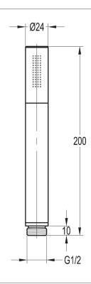
Dimensions are in millimetres except thread sizes which are BSP imperial.
