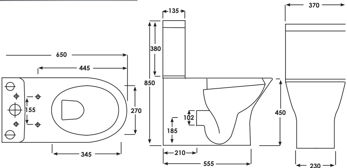
Dimensions: All measurements are in millimeters and are subject to normal manufacturing variations.
