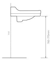
Ensure the basin is firmly screwed to the wall using appropriate basin fixings before proceeding. Fix the basin in accordance with the fixing manufacturer's instructions.
