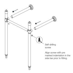
Centrally align the washstand and adjust the extension appropriately.
