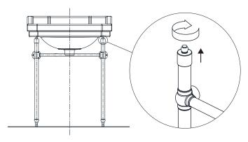
Once the washstand is aligned and level, mark out and drill the pilot holes. Insert the wall plugs and using the screws provided attach the washstand to the wall
