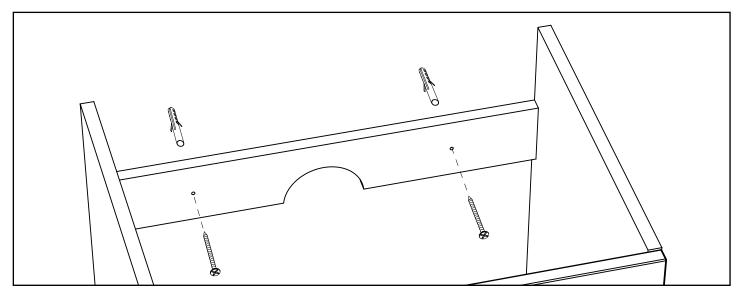
It is recommended to secure floor mounted units to the wall, this can be done by using a screw and wall plug as shown above (fixings not supplied).
