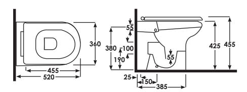
Dimensions: All measurements are in millimeters and are subject to normal manufacturing variations.
