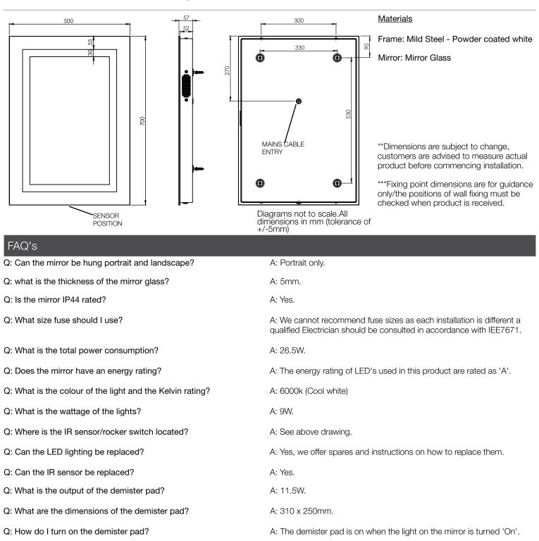
All Illuminated mirrors are supplied with approximately 500mm of mains cable. This can be removed for the customer to make their own connection to their mains supply. There is ample storage for excess cable in the back of the unit.
