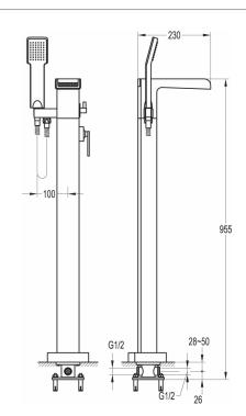
Dimensions are in millimetres except thread sizes which are BSP imperial.
