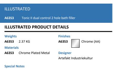
Suitable for balanced or unbalanced supplies. Inlets with G3/4" connections.
