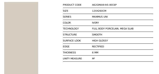
Dimensions: All dimensions in mm tollerance +5% for below 200mm and +3% for above 200mm.
