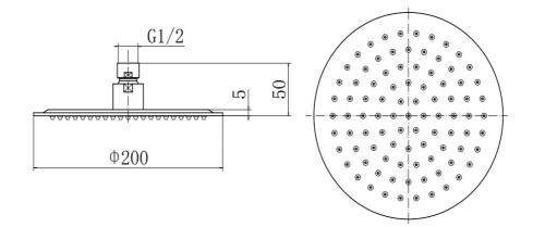
Products are supplied with full installation instructions and fixings. All measurements in mm and are nominal.
