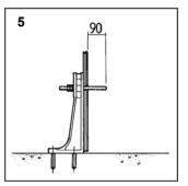
Assemble nuts and washers onto studding so that studding protrudes 90mm from front of panel. Nuts should then be locked tightly together.
