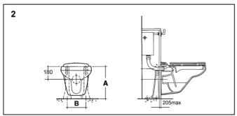
Normal height of w.c. basin (dimension A) is 400mm. Design of floor brackets also allows heights of 375mm, 425mm or 450mm.
