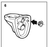
Fit flushbend seal provided into w.c. basin.
