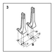
Drill holes for floor brackets as shown. Secure brackets to floor using M12 rawlbolts (not supplied).
