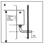
Fix cistern at maximum height shown above. Install cistern as per the instructions provided
