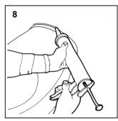
Seal around back and sides of w.c. with silicone building sealant.
