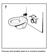
and fit w.c. basin onto studs. Secure basin in position using fixings and instructions supplied with the w.c.
