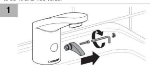
Remove hot water limiter from mixer handle using pliers, turn it by 180°, and insert it again. Push O-ring into second groove.
