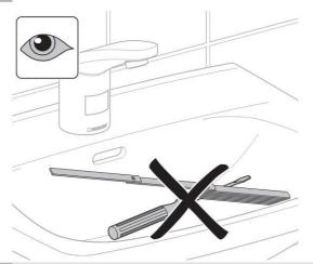
Cover the IR window completely with your hand. Water will stop after 5 s. Wait until 4 further water impulses have occurred.
