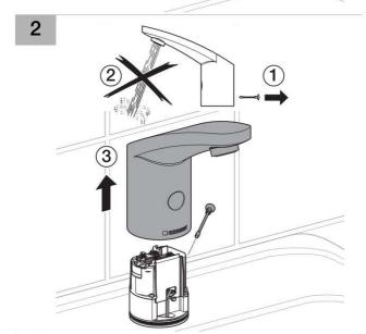
Remove dead battery and dispose of it appropriately.
