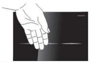
3 Cover the actuator button on the left with your hand again until it lights up yellow. The actuator button on the right flashes repeatedly to show the current setting 1 or 2 (flashing once = setting 1, flashing twice = setting 2).
