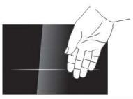
Cover both actuator buttons at the same time with your hands at a distance of approx. 5 cm until both actuator buttons flash once.
