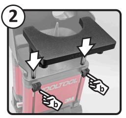
a) Slide the PLATFORM assembly into the JOOLTOOL's post holes **b)** Install the KNOBS loosely. Do NOT tighten them yet.
