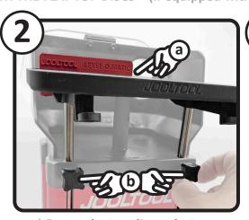
a) Ensure the Leveling tab sits flat on the FLAT TOP DISC
