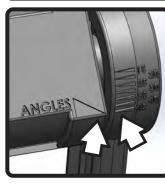
set the desired angle by aligning indicators on **RIGHT-HAND** post with the ANGLES indicator.
