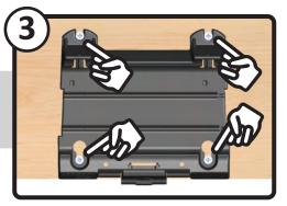
Set the BASE close to edge of bench or table and secure with screws of your choice. Refer to 4 locations shown above. If setting on a glass surface, use the pre-installed rubber "feet" at all 4 corners of the base.
