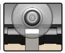
Always make uniform contact with the spinning abrasive. Use coarse abrasives to re-grind edges and fine abrasives to polish. When done, slide the Chisel away from the disc and turn the JOOLTOOL OFF. SEE DEBURRING INFO ON NEXT PAGE
