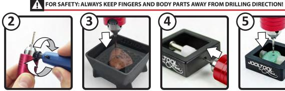
Using the chuck key, tighten the jaw. Note: Check if the bit is centered by rotating the chuck by hand.
