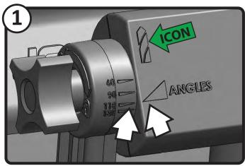
Rotate the main PLATE to the DRILL BIT side (ICON). Set the desired angle by aligning indicators on LEFT-HAND post with the ANGLES indicator. The most common setting is 118 degrees Lock with LOCKING KNOB.
