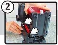
Set the Jooltool to its side and align the Holes at the rear of the Tool with the ALIGNMENT PINS on the BASE. Speed control switch will be pointing upward when properly docked.
