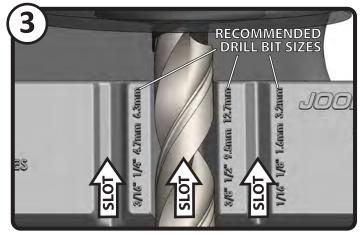
Select the guide slot of corresponding Bit diameter. Sizes shown next to SLOTS are recommendations. Slide the drill bit into the spinning disc. Ensure a secure, flat contact with the full length of the slot.
