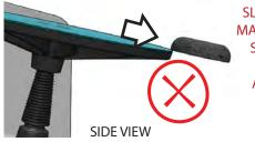
SLIDING OFF THE DISC MAY CAUSE UNWANTED STRIATIONS ON THE FINISHED PIECE AND MAY DAMAGE YOUR ABRASIVES
