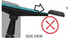
SLIDING OFF THE DISC MAY CAUSE UNWANTED STRIATIONS ON THE **FINISHED PIECE** AND MAY DAMAGE YOUR ABRASIVES
