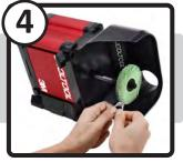
This is a classic, bench style of polishing and finishing. NOTE: The Vacuum Port is fully functional in both Horizontal & Vertical modes.
