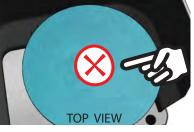
WORKING IN THE CENTER PORTION OF THE DISC MAY CAUSE INSTABILITY, UNEVEN FINISHES AND MAY PREMATURELY WEAR **OUT YOUR ABRASIVES**
