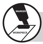
ANIE'S TIP: To improve visibility of the surface or edge you are working on, darken it with a black marker (Sharpie<sup>™</sup>) or use a marker color that contrasts with the surface to be worked. The marker gets erased on contact with the abrasive.
