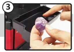
The drawer/water tray can hold water for quick access to lubrication when performing lapidary work.
