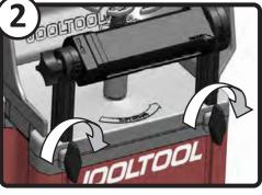
Lock the Tool Rest in place by tightening the post locking screws (Turn Clockwise to lock)
