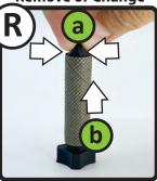
Use Step **2.2** to remove mandrel from Spindle
