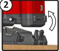
Press EJECT BUTTON to release the tool from base.
