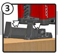
Slide machine away from ALIGNMENT PINS to fully detach from docking base.
