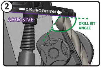
The resulting **drill bit angle** will be as set in STEP 1. Use coarse grade abrasives such as 3M Purple Ceramic to regrind damaged bits. Use 3M Trizact<sup>™</sup> for honing edges. **Tip: Use 3M Diamond Abrasives for Carbide Bits.**
