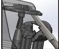
Sharpen the Chisel by sliding the cutting edge it into the spinning disc. Use coarse grades such as 3M Purple Ceramic for regrinding a damaged edge. Use fine grades (3M Trizact™)
