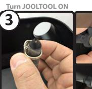
Turn the JOOLTOOL ON and enjoy quick and easy grinding, sanding and polishing inside rings, stones & more. **Note:** Mandrel can also be used while in Horizontal Mode. (p.13) GRIND
