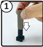
Slide the abrasive tube of your choice onto the mandrel, starting from the tip.
