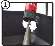
Slide the Flexshaft Connector Hub onto the Jooltool spindle. This is similar to installing Backpads onto the Spindle.
