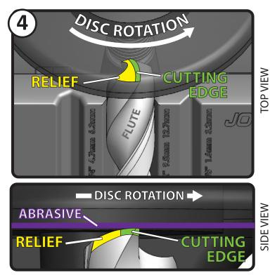
Rotate the drill bit on its main axis to sharpen all CUTTING EDGES. Make sure each cutting edge is higher than its RELIEF. (back of the flank). This will ensure the bit cuts well and extracts drilled material properly. Slide the bit along the slot, away from the disc and turn the JOOLTOOL OFF when done.
