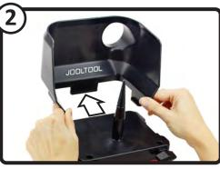
Slide the Hood out and away from the Jooltool. Reverse steps 1 & 2 to reinstall (Center the rear tab, pull towards you, snap tabs back into their slots)
