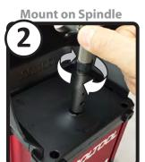
2.1) Twist clockwise onto the Spindle of the JOOLTOOL using grip areas at the bottom of the mandrel.
