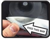
FIND THE EDGE ANGLE (as shown in STEPS 1-2 above), then GRADUALLY FEED the workpiece's edge under the disc while keeping a FULL and FLAT contact. Work from the inner to the outer edge. You may stop anytime by simply lowering the workpiece as described above in STEP 3.
