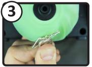
Use FULL speed. Apply workpiece to the OUTER EDGE with light pressure
