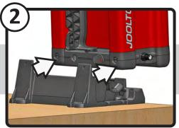
(.1) Slide machine off ALIGNMENT PINS to detach from BASE DOCK
