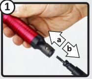
a: Insert the Flexshaft's Paddle (Key) Tip into Handpiece until it snaps & locks in place. b: To remove: Pull apart
