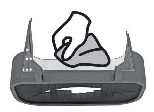
DO NOT use harsh chemicals or abrasive pads to clean your GRIND GUARD and acrylic visor.
