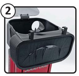
Ensure the GRIND GUARD is secure and it meets the HOOD of your JOOLTOOL on all sides.
