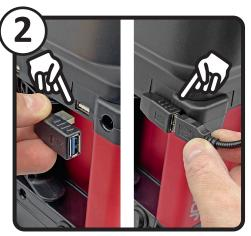
Insert the Right-Angle USB adapter into your rear USB port, then connect the USB Light to it.
