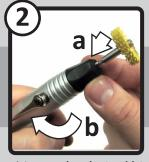
a) Insert the desired bit b) reset the lever in-line with Handpiece to close & lock.
