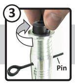
Insert & screw on the collet nut but do NOT tighten yet.
