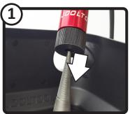
Slide the Flexshaft Connector Hub onto the Jooltool spindle. This is similar to installing Backpads onto the Spindle.
