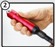
Once installed, test run the JOOLTOOL at various speeds. Rotation should be smooth. If vibration occurs, turn JOOLTOOL off and re-install.
