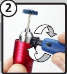
Using the chuck key, tighten the jaw. Note: Check if the bit must be opened wide is centered by rotating
