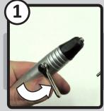
Position the locking lever perpendicular to Handpiece. This opens the chuck.
