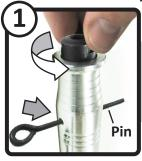
Insert pin into the Handpiece. Unscrew & remove the collet nut. Use wrench if needed.
