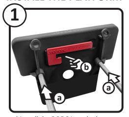
a) Install the RODS into the bottom of the PLATFORM as shown.b) Locate the Leveling tab for later use (see below)
