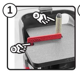
a) Install the SANDING MANDRELb) Snap the Leveling tab into the left notch on the PLATFORM.
