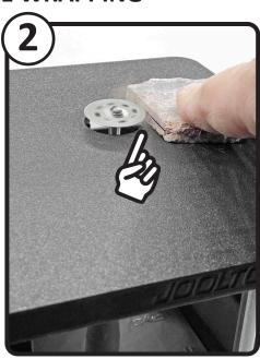
Set the platform at a low setting and Adjust the PLATFORM height as needed for Wire-Wrapping.
