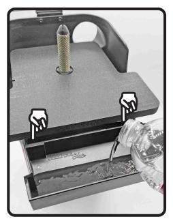
Use with the WATER TRAY for convenient access to lubrication. It attaches to the two eyelets located under the PLATFORM.
