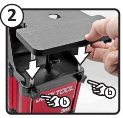
a) Slide the PLATFORM assembly into the JOOLTOOL's post holes
