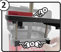
a) Ensure the Leveling tab sits flat on the base of the Mandrel.
