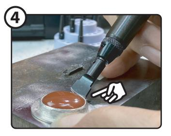
USE THE ANVIL TIPS at any desired speed setting of your JOOLTOOL MACHINE. The Reciprocating motion does the work; you simply guide the tip as needed.
