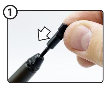
INSERT THE ANVIL TIP into the receiving hole of the HAMMER HANDPIECE
