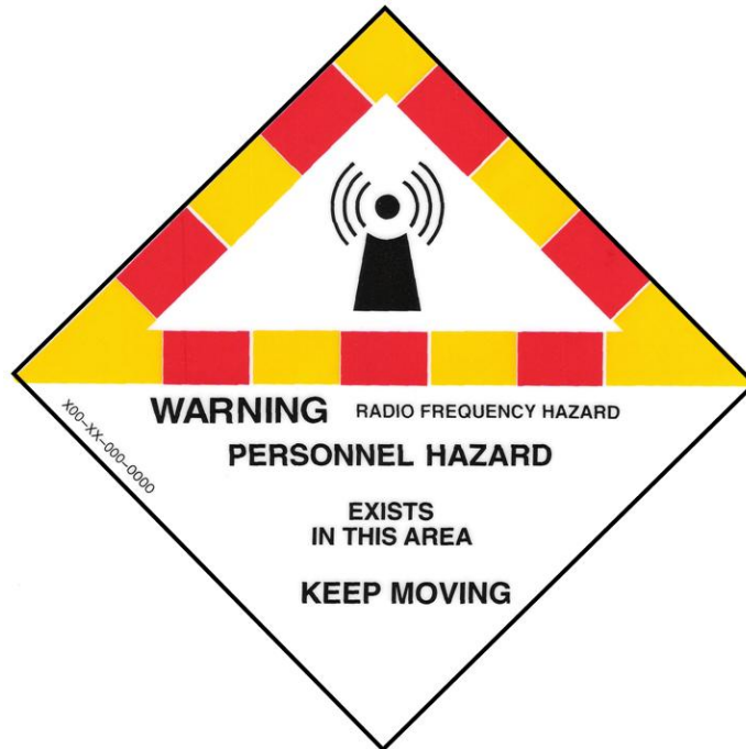
Figure 10-2. Current RF alerting sign example used within the US Department of Defense.
