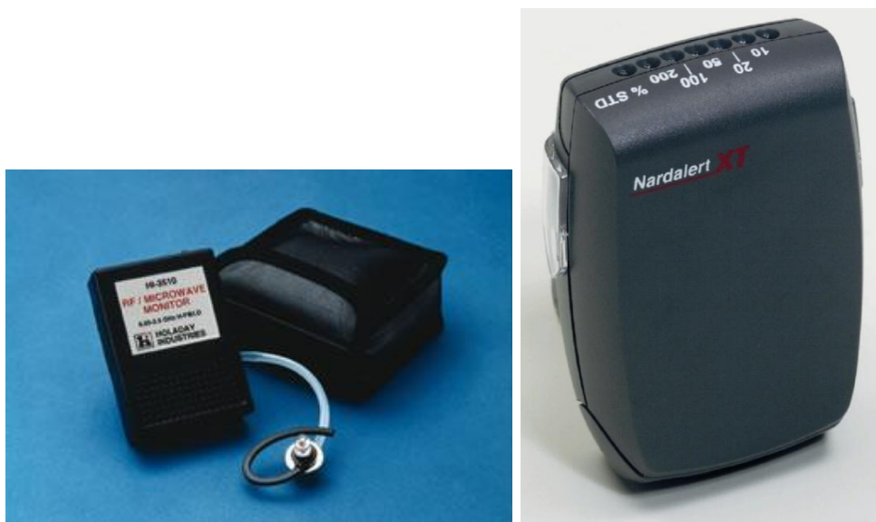
Figure 9-9. Typical RFR personal monitors (Drawings courtesy of Holaday Industries and L-3 Communications, NARDA East).
