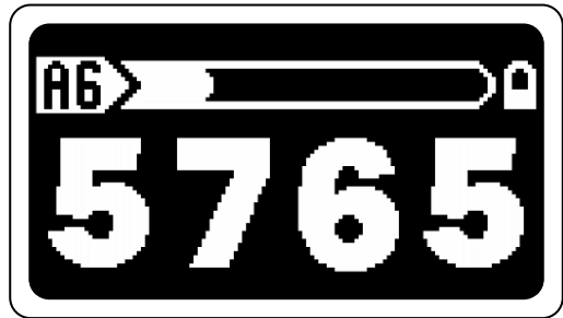
When "Channel Lock" is ON, the home screen interface will display a lock icon.
