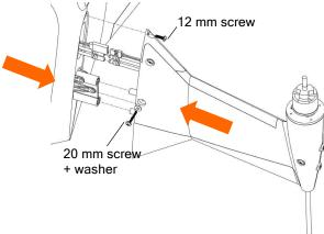
\*if there is resistance, "hug" the pylon to the craft by placing the motor mount in the pit of your arm and squeezing the pylon into place with your hand.
