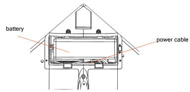
c) Cover the battery and all wires with the battery cover.
