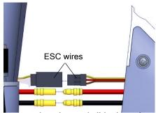
b) Insert the pylon spars into the connector on the wing and slide the pylon onto the wing. Bundle the wires into the cavities in the wing and pylon.
