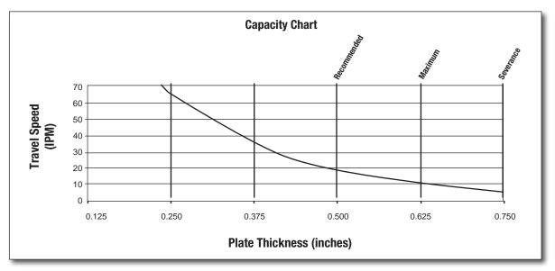
Aluminum cutting speeds are typically 10-20% faster than mild steel.
