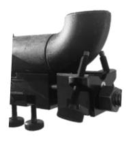
A bolt on saddle attachment (easily installed and removed), that allows for the quick adaptation of the QFIII clamp to quickly accommodate various fittings from 1 to 10in. The 2 jack screws provide the ability to quickly adjust and level various fittings and sizes.
