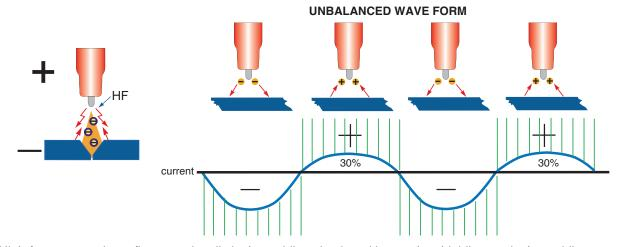
High-frequency voltage flows continually in the welding circuit and keeps the shielding arc in the welding area in an ionized state. When the arc is ionized the arc is maintained during the half of the cycle when the electrode is positive. However while the arc is maintained less current flows during this half of the AC cycle, producing an unbalanced wave.
