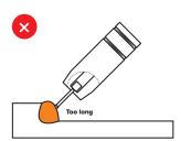
Unstable arc, spatter, poor penetration and fusion.
