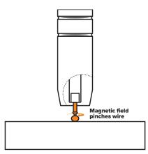
The current flow creates a magnetic field that begins to pinch the melting wire forming it into droplet.
