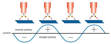
A square wave power supply can change the current from electrode + positive to electrode - negative very quickly. This produces high voltage as the current switches polarities allowing the arc to restart easily. The arc can be maintained without the use of high-frequency or any other arc stabilising methods.
