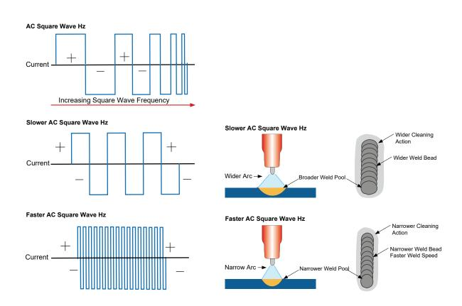
AC (alternating current) enables us to TIG weld non ferrous alloys like Aluminum, Magnesium and Aluminum Alloys. These materials have an insulating surface oxide layer that melts at a higher temperature than the base metal making it difficult to weld the base metal if the oxides are not removed. AC welding current is ideal because the nature of the AC wave form assists in breaking the surface oxide layer.
