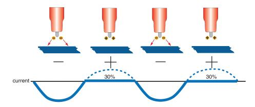
To overcome this lack of flow during one half of the cycle, a high-frequency (HF) voltage is generated and fed into the welding circuit. The HF maintains the arc stability during the half cycle when the electrode is positive.
