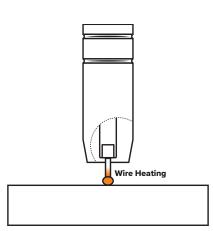
An arc is created at the separation of the droplet and the heat and force of the arc flattens out the droplet into the weld pool. The heat of the arc melts the end of the wire slightly as it feeds towards the base metal.
