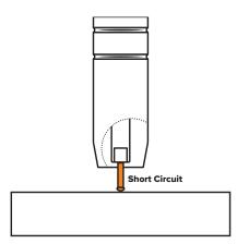
The wire approaches the workpiece and touches the work, creating a short circuit between the wire and the base metal, because there is no space between the wire and the base metal there is no arc and current flows through the wire.
