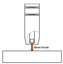
The pinch causes the forming droplet to separate and fall towards the forming weld pool.
