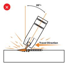
Poor control, unstable arc, less penetration, lots of spatter.
