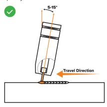
Good level of control over the weld pool, even flat weld.
