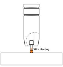
The wire cannot support all the current flow, resistance builds up and the wire becomes hot and weak and begins to melt.
