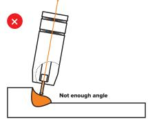
Less control over the weld pool, more spatter
