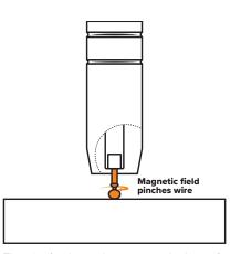
The wire feed speed overcomes the heat of the arc and the wire again approaches the work to short circuit and repeat the cycle.
