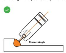
Good level of control over the weld pool, even flat weld.
