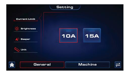
Select the **Settings** menu from the Home Screen. Press the **Right Action Button** to cycle between the **General Settings** and **Machine Settings** menus.
