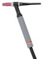
PTA-26, PTA-26V, PTA-26F and PTA-26FV Air-cooled TIG torch, rated 200 amps at 60% duty cycle. The PTA-26V is equipped with a valve for gas flow control. The PTA-26F is equipped with a flexible head for easy maneuverability into tight spaces. The PTA-26FV is equipped with both a gas valve and flexible head.
