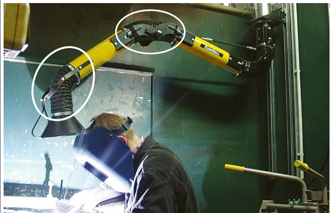
Exterior friction joints ("ClearThru" design), which allows for maximum air velocity, low pressure drop and low noise level
