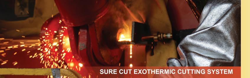
The Sure Cut Exothermic Cutting System will cut virtually any metal, both ferrous and non-ferrous, and it is faster than conventional oxy-acetylene or carbon arc gouging. Exothermic cutting requires no preheating or cleaning the material prior to cutting. It is easy to use and is cost effective for most applications. Unlike carbon arc gouging, the Sure Cut System leaves no carbon residue on material being gouged.
