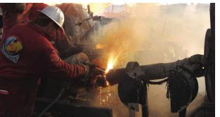
**FOUNDRIES, STEEL MILLS AND SCRAP PROCESSORS**: removing risers, opening tap holes cutting up scrap and equipment maintenance.
