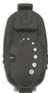
Control module with push button on/off switch with roller potentiometer.
