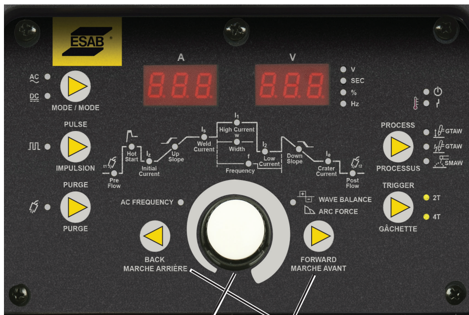
Art# A-13116 Adjust programming parameter Press to go forward / go back between programming status LED's
