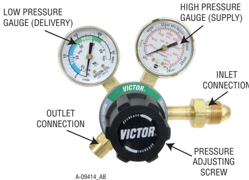
Figure 3-7: Victor CS Regulator
