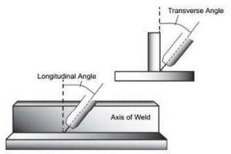
Transverse and Longitudinal Nozzle Axes
