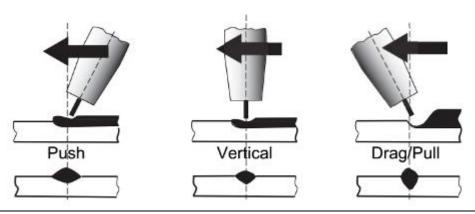
The welding gun should be held at an angle to the weld joint. (See Secondary Adjustment Variables below) Hold the gun so that the welding seam is viewed at all times. Always wear the welding helmet with proper filter lenses and use the proper safety equipment.
