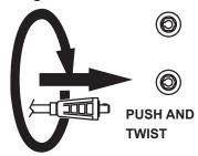
Connect the earth clamp to the negative pole and the electrode holder to the positive.
