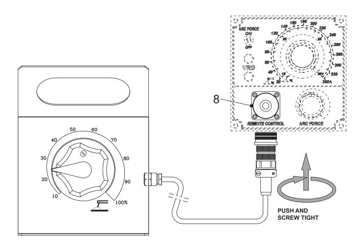
The remote control device for regulating the welding current is connected to the front panel by means of a multipole connector.
