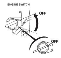
Turn the fuel valve to the OFF position.
