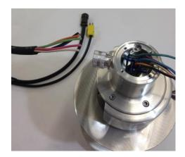
Gently bring the wires out with the needle nose pliers, cut them all to the same length and strip the insulator on all the wires as shown.
