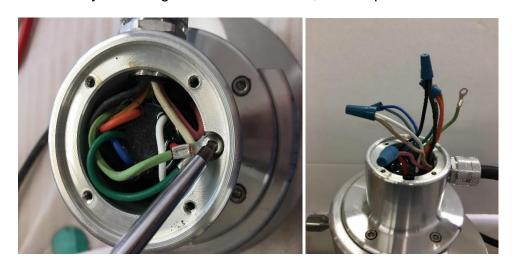
Loosen the nut on the wire connector using the adjustable pliers. Pull the existing cable out of the connector and discard. Gently feed the new pigtail you've made from your welder remote cable into the connector until the jacket is in line with the inside wall of the junction box and retighten the connector.
