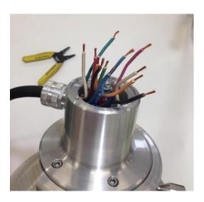
Connect the wires by twisting the copper conductors and securely installing a wire connector on each pair. Reconnect the ground wires using #8 screw and eye terminal **Be sure to match the colors correctly. Always double check.** There is enough room to tuck the wires neatly into the junction box, do not force or compress.
