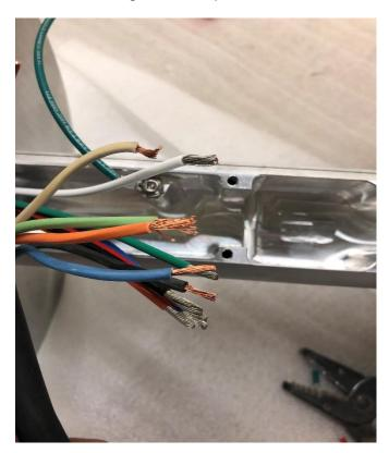
Connect the wires by twisting the copper conductors and securely installing a wire connector on each pair. Connect all the green wires together (green wire on shaft, green wire from remote cable, and green wire coming from reel mount) **Be sure to match the colors correctly. Always double check.** There is enough room to tuck the wires neatly into the junction box, your remote wire should run nicely in the grove towards the end disk, do not force or compress.
