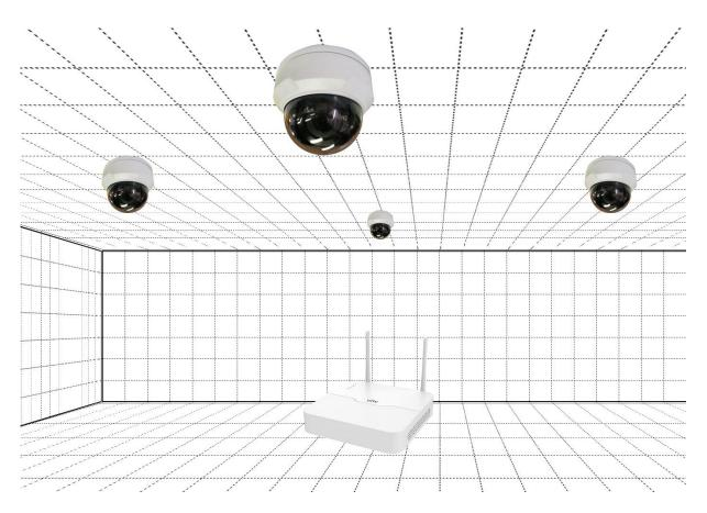
When installing the Wi-Fi dome, NVR should be placed below the dome. It is not recommended to place the NVR above the dome.
