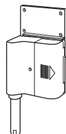
When the detection rod is fully extended, the receiver will beep and zone LED will flash.
