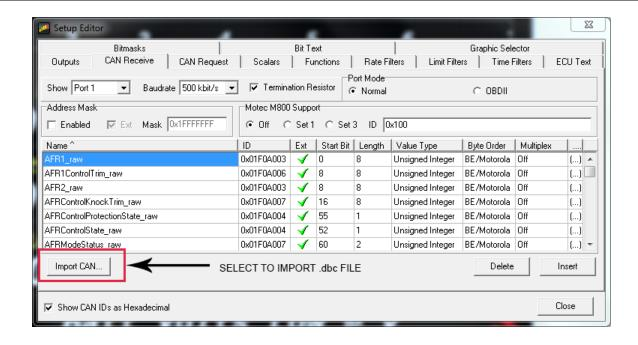
The "Start Bit" refers to the location of the LSB. The message contents and the byte/bit numbering can be viewed by clicking on the ... button for each message.
