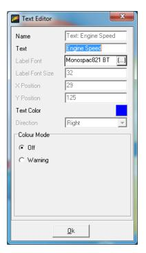
The dialog allows editing of all unlocked characteristics if Layout Locked is turned on. Locked characteristics are typically related to size and position. To change the text displayed in the text label example above, simply highlight the text and edit. Double clicking on the "0" in the example above opens the value label editor. This is live data displayed on the screen.
