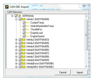
Select the channels for import by clicking the boxes. All available channels are selected by default. Click the Import button to import. All CAN message information is automatically imported along with necessary Scalar and Bit text operations. The channels are now available for assignment.
