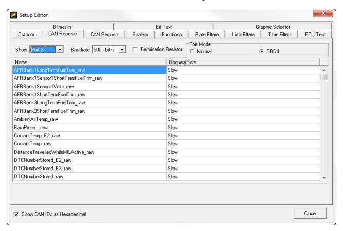
This is a complete listing of available PIDs. An AEM supplied setup file for OBDII messages will be located in the \Documents\AEM\DashDesign\Setups folder. The basic default OBDII file is named Default-Black-OBD2.aemcd7.
