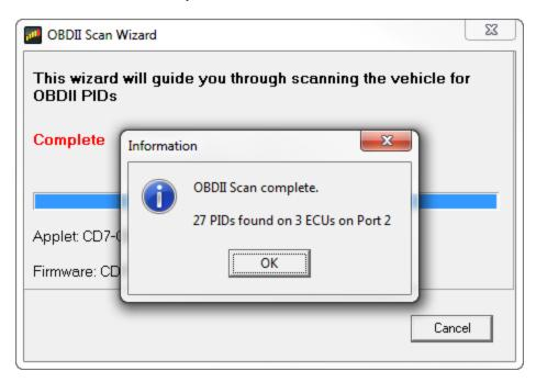
The scan is complete. Click OK. You can now disconnect the USB cable. Your dash will reboot to complete the process.
