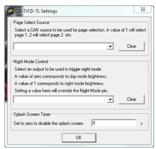
The Settings dialog will be populated correctly with all AEM supplied setup files. The options can be changed for custom setups. Night mode dialog box should be empty unless you want to control the mode via CAN. Default is empty and controlled by the flying lead harness input.
