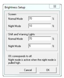
The Brightness setup dialog allows you to choose two different brightness settings for both the screen and LEDs. See CD-7 Harness and Wiring section for Night Mode input wiring. 100% should only be used in direct sunlight. 70% gives almost as much brightness without overdriving the backlight. 5%-10% is appropriate for night mode.
