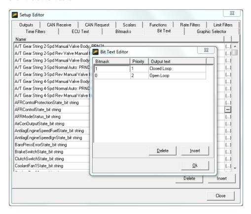
The priority determines the order in which the bitmasks are evaluated with low numbers being a higher priority. This ensures that if two bitmasks match, only the highest priority output text is returned from the sensor.
