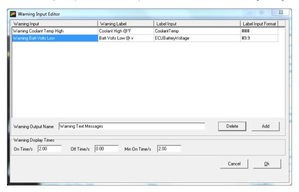
The example above shows two existing Warning Inputs. These were both previously defined as Alarm outputs before setting up this window.
