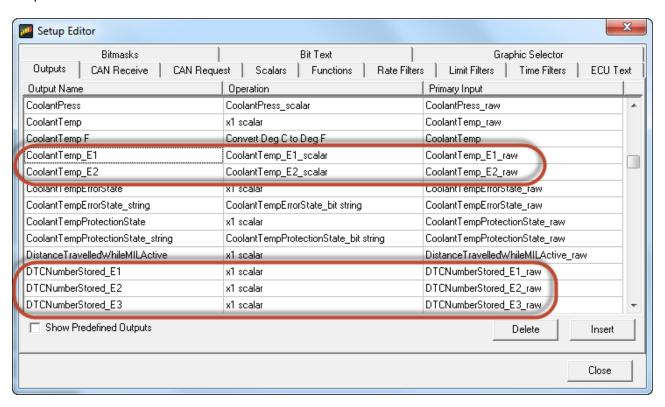
Open the Setup Editor. OBDII PIDs will be automatically added to your list of available outputs. The circled examples above represent the same PID from different vehicle ECUs. In these cases, the system will append a suffix. E1 for ECU1, E2 for ECU2, etc. These outputs are now available for use as inputs to gauges for
