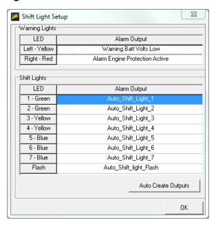
The LED and shift light setup will be pre-configured with AEM supplied setup files. The Alarm outputs used to trigger the LEDs can be adjusted in the Setup Editor as shown in the example below.
