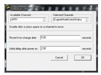
The example below shows one version of an AEM supplied On Change Page. Different operating modes and/or multi-map selections can be displayed using this page. Other useful items are boost target and traction controls set points.
