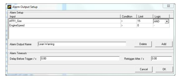
Above, the input EngineSpeed is added as an "AND" condition with a limit of 0 RPM. With this logic, IF AFR1\_Gas is greater than 15 AND EngineSpeed is greater than 0 (engine running), the alarm will trigger.
