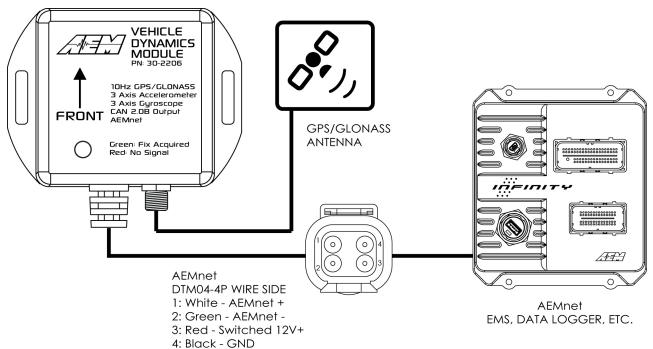
The VDM is equipped with an AEMnet connector (power, ground, and CAN) so that it is a true plug and play experience when used with other AEMnet products such as the Infinity ECU.
