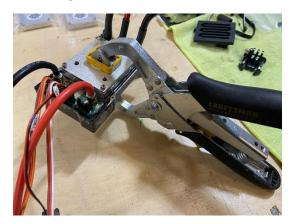
Step 7: If you used thermal grease you will need to secure the cooler to the ESC. You can use thick zip ties or strong tape wrapped around the ESC and cooler to secure it.
