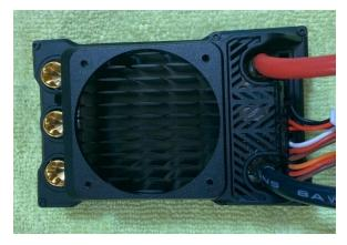
Step 2: Remove the 6x- screws around the periphery of the fan shroud using a 1.5mm Allen wrench.
