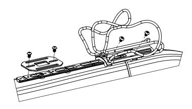
**STEP 4.** Tighten frame screws to manufacturers recommended torque (See notes). Check clearances with bottle cage and accessories installed before riding.
