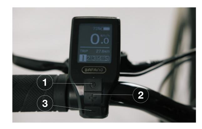
To power on the ebike, locate the Power button (1) and hold for a few seconds until the display turns on.
