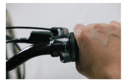
To shift gears upwards, ensure your pedals have stopped spinning and twist the shifter towards the "+" symbol, in a downwards motion.
