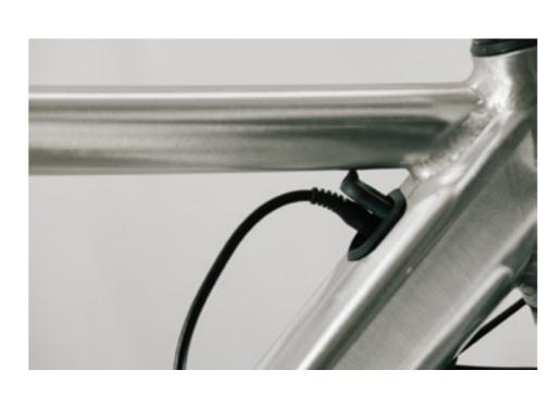
Once the charger jack is securely inserted into the charging port, turn the charger on at the power point to begin charging.
