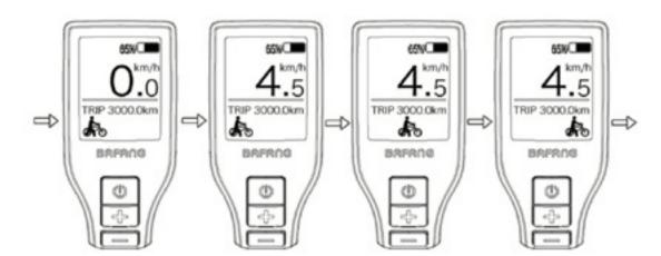
Walk Assist can only be activated when the ebike is at a standstill. To activate hold the DOWN button until the walk assist icon appears. The icon will flash and the ebike will move at 6km/h. Releasing the Down button will stop the motor automatically.
