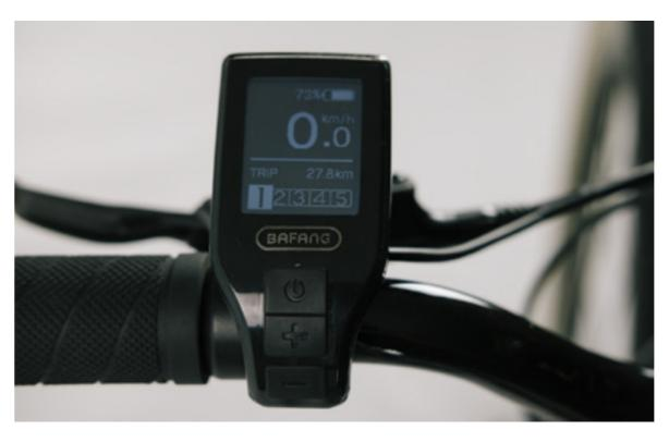
By the left grip on the handlebar you will find the display and integrated 3 button keypad that controls the ebike power system.
