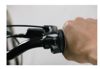
To shift down a gear, ensure you have stopped pedalling and twist the shifter towards the "-" symbol, in a motion upwards and away from you.
