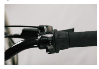
Your Miller ebike is equipped with an internally geared hub and a handlebar twist shifter allowing you to change gears up and down.
