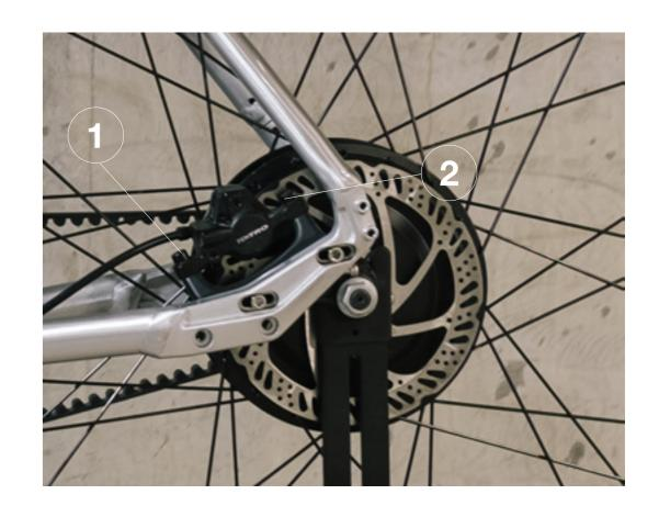
Rear brake caliper positioning adjustments and removal can be accessed via bolts (1) and (2) above with an allen wrench.
