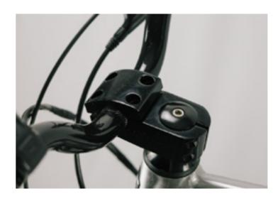
Replace the previously removed top piece and install the four bolts by hand to ensure correct installation.
