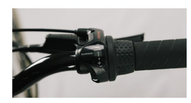
By the right grip on the handlebar you will find the twist shifter allowing you to shift gears up and down.
