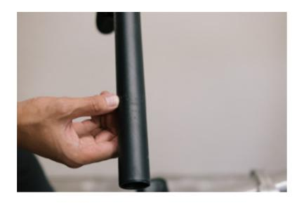
When raising the seat height, ensure that you do not extend the seat height past the minimum insertion point marking on the seat tube.
