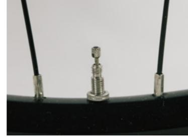
Attach a presta valve compatible tire pump and inflate to the desired pressure.
