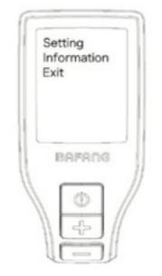
After the display is turned on, press the UP and DOWN button at the same time (>2 s), to access the "PROP-ERTIES" menu. Via this menu you can further select: "Setting", "Information" or "Exit". Then press the POW-ER button (<0.5 s) to access your selected option.
