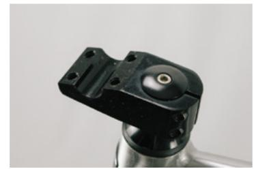
Using a 6mm allen wrench, undo the four bolts at the top of the head stem and remove the top piece.
