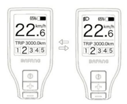
Hold the Up (>2 s) button to turn on the headlight and display backlight.
