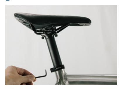
To adjust the seat height, locate the seat post clamp at the top of bicycle seat tube and insert the allen wrench. Loosen the clamp by turning the securing bolt in an anti-clockwise direction until the seat post moves freely up and down.
