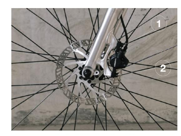
Front brake caliper positioning adjustments and removal can be accessed via bolts (1) and (2) above with an allen wrench.
