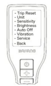
From the PROPERTIES menu press the UP or DOWN button (<0.5 s) to select "Setting", and then briefly press the button (<0.5S) to access the following options:
