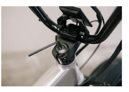
Straighten the handlebar so that a forward facing handlebar coincides with a forward facing front tire, then secure by removing the rubber cover and tightening the top cap bolt.
