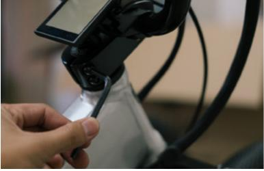
Adjust the display position so that it can be easily viewed when sitting on the bike, then finally secure the handlebar by tightening the two pinch bolts using an allen wrench.
