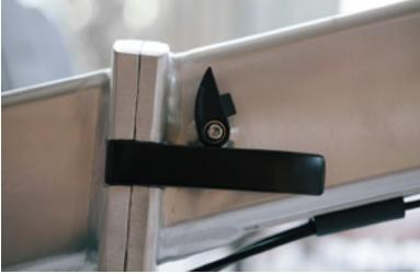
Rotate the lock clasp anti-clockwise so that the locking tab that sits inside the hole of the clamp lever handle no longer secures the clamp lever handle in place.
