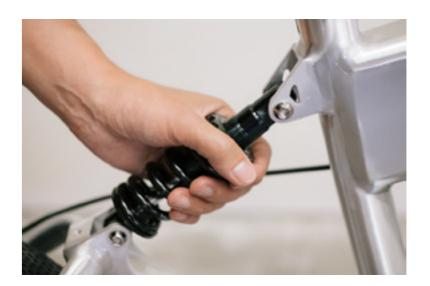
Twisting the stopper in an anti-clockwise direction reduces the amount of preload.
