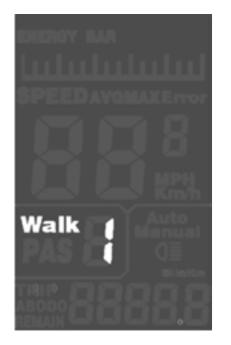
Pressing the Down button for 3 seconds activates the "Walk mode", where the ebike will travel at a constant speed of 6km/h.
