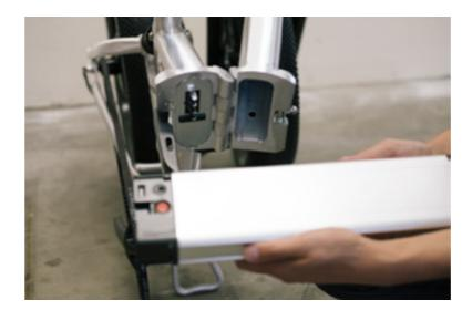
Slide the battery out completely and charge in a cool dry location until fully charged.
