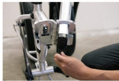
Ensure that the ebike's power button is switched to the off position (0).
