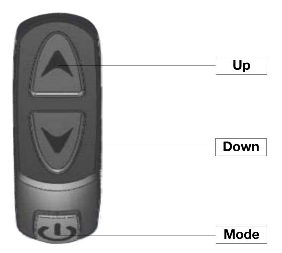
To power on the ebike, hold down the Mode button for a few seconds until the display turns on.
