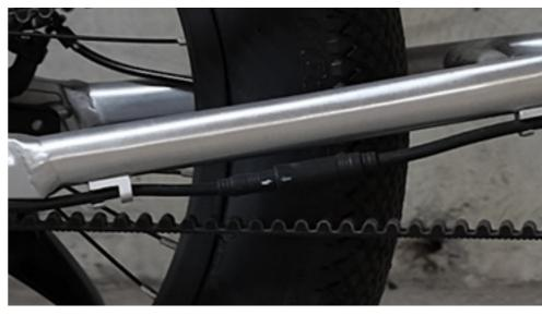
Ensure the motor cable is securely connected to the controller connector cable.
