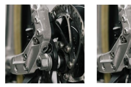
Next, locate the setting screw via the hole at the rear of the silver dropout arm, just above the main axle nut.
