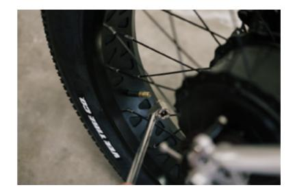
Attach a schrader valve compatible tire pump and inflate to the desired pressure.
