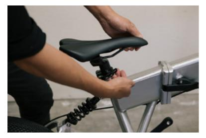
Seat adjustment is achieved without tools via the quick release system. To adjust, locate the quick release lever at the top of the seat tube. When raising the seat height, ensure that you do not extend the seat height past the minimum insertion point marking on the seat tube.
