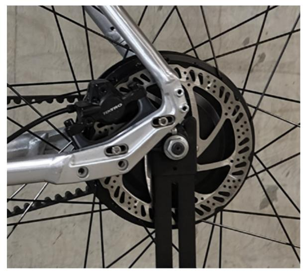
Your Billy ebike comes equipped with front and rear hydraulic disc brakes, designed to help you slow down and stop as required.
