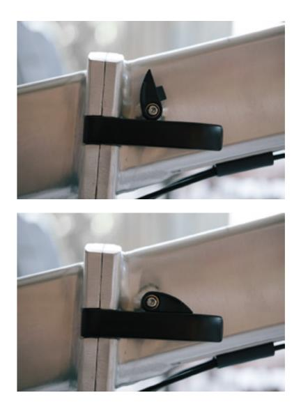
Rotate the lock clasp clockwise so that the locking tab sits inside the hole of the clamp lever handle and the lock clasp sits flush against the handle.
