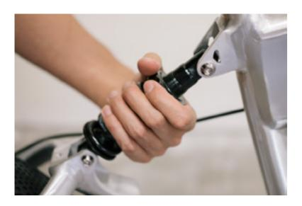
Twisting the stopper in a clockwise direction increases the amount of preload.
