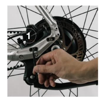
Your rear wheel axles are secured into the black dropouts via an 18mm nut. The belt tension and wheel alignment are set by adjusting the floating black dropouts either forward or rearward as required.
