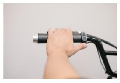
By the left grip on the handlebar you will find the 3 button keypad that controls the ebike power and display system.
