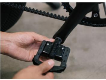
Next, locate the right side crank and attach the pedal to the arm by threading in a clockwise motion.
