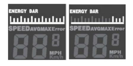
When fully charged, the energy bar across the top right of the display will show bars spanning the width of the display.
