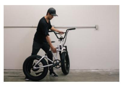
Slowly swing the handlebar half of the bike outwards in a motion that closes the center hinge.
