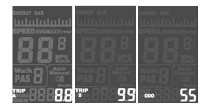
Pressing the Mode button also cycles through the various trip and odometer readings of the display. Pressing Down and Mode simultaneously resets displayed trip meter.
