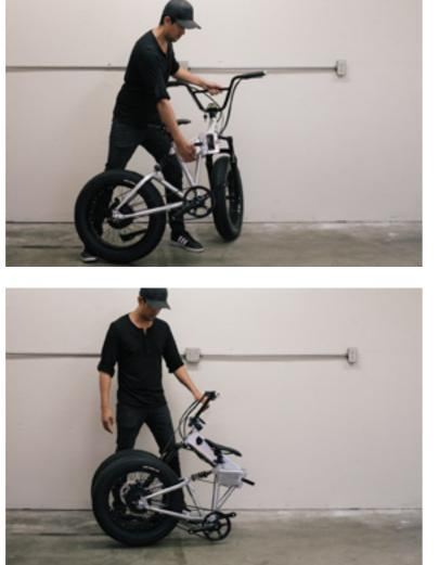
With an anchoring foot behind the rear wheel to stop it from rolling backward as you fold, use one hand to hold the frame close to the seat post and the other hand to hold the front half of the bike. Fold the bike in half using a swinging motion, until the front wheel aligns with the rear wheel. Allow the bike to rest on the lower guard for storage with a smaller footprint.
