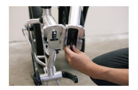
To charge the battery away from the ebike, fold the bike in half and use the supplied key to unlock the battery from its mounted position.
