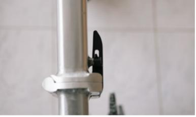
Clasping the clamp lever handle, draw it closed by swinging it across the frame break so that there is an even gap between the lever handle and the front half of the frame. It is designed to sit very close to the frame, but not actually touch it.
