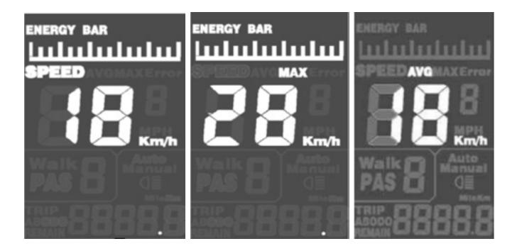
When powered on, pressing the Mode button will cycle through the various speed interfaces of real time speed, average speed and maximum speed.
