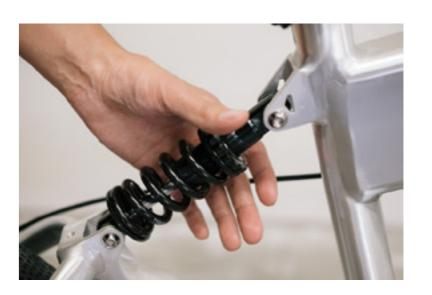
To adjust, locate the textured threaded stopper that sits at the end of the suspension spring, towards the top of the rear suspension unit.
