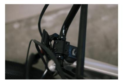
Just before the bolts are fully tightened, adjust the handlebar so that the vertical bars are in line with the forks and the brake levers face forward.
