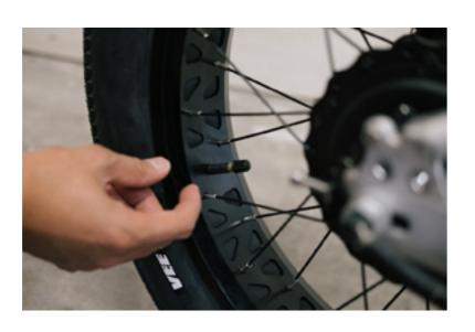
To inflate, locate the inflation valve on the tire.
