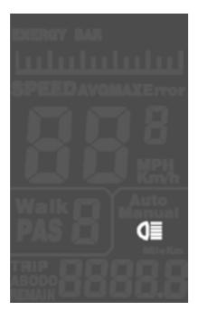
Pressing the Up button for a few seconds illuminates the display for viewing ease when lighting conditions are low. Once illuminated, pressing Up again for a few seconds returns the display to the standard non-illuminated view.
