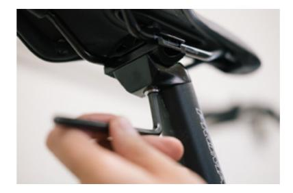
To adjust, loosen the securing bolt with an allen wrench and turn in an anti-clockwise direction.
