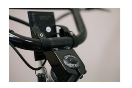
Pointing the handlebars with the levers facing down, place the knurled center section of the bar in mounting point of the head stem.
