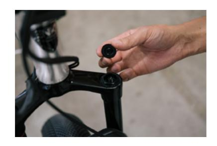
Remove the "Air" cap by turning in an anti-clockwise direction and inflate using a high-pressure air suspension pump. Recommended starting pressures are listed below based on rider weight.
