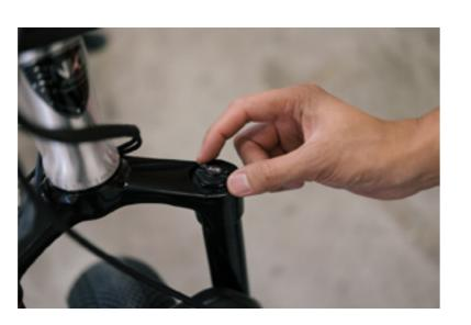
It is also possible to adjust the amount of preload on the air suspension.
