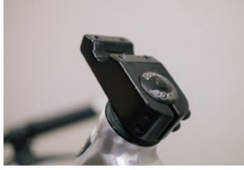
Using a 6mm allen wrench, undo the four bolts at the top of the head stem and remove the top piece.
