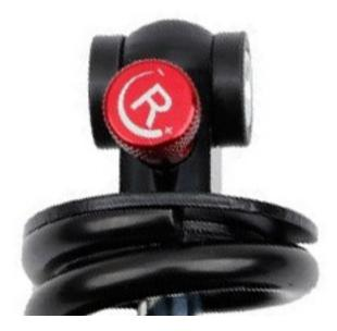
The rebound damping dial determines the rate of return when the shock is compressed. Full clockwise will set a slow rate of return and anti-clockwise for incrementally faster return.
