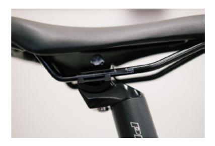
Once the bolt is loose enough, there should be enough play in the seat rail clamp to allow the seat to slide back and forth. Ensure that you only slide the seat so that the seat rail clamp's edges sit within the range marked on the seat post rails.
