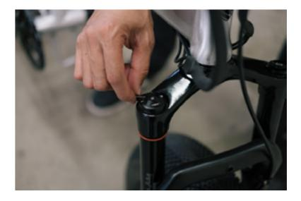
Billy's suspension fork features a lock out dial. When fully locked out (the lock icon on the dial is closest to the frame), the fork will be fully rigid, meaning it will ride like a standard rigid fork bicycle.
