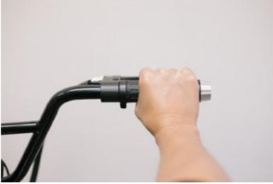
**USA MODELS ONLY:** The right side grip is a motorcycle style twist throttle. Twisting the grip down towards the rider dictates the level of throttle applied. Brake lever positioning varies from region to region. While we officially ship correct configurations to regions, It is important to understand which regional versional version you have so that you know which lever controls which brake.
