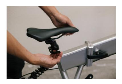
Open by pulling towards the rear of the bike. The seat post should now be loose enough to adjust the seat height.
