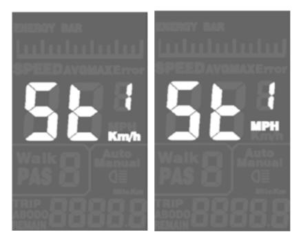
The first setup option allows you to switch between imperial (miles) and metric (kilometres) forms of measurement by pressing Up or Down. Confirm your selection by pressing Mode and return to the setup menu. 522
