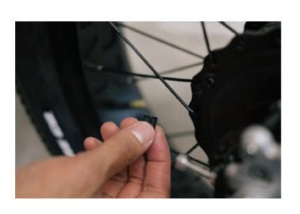
Remove the valve cap by twisting in an anti-clockwise motion.
