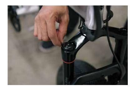
Billy's suspension fork features a lock out dial. When fully locked out (the lock icon on the dial is closest to the frame), the fork will be fully rigid, meaning it will ride like a standard rigid bicycle.
