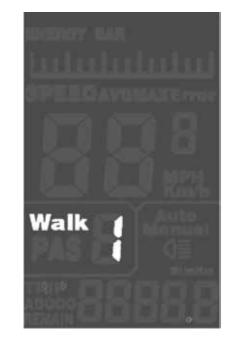
Pressing the Down button for 3 seconds activates the "Walk mode", where the ebike will travel at a constant speed of 6km/h.
