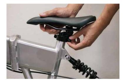
If the seat post is loose when the quick release is fully engaged it may be necessary to adjust the clamp further to secure the seatpost correctly. This is achieved by turning the adjustment dial clockwise when the clamp is released.
