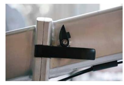
Rotate the lock clasp anti-clockwise so that the locking tab that sits inside the hole of the clamp lever handle no longer secures the clamp lever handle in place.
