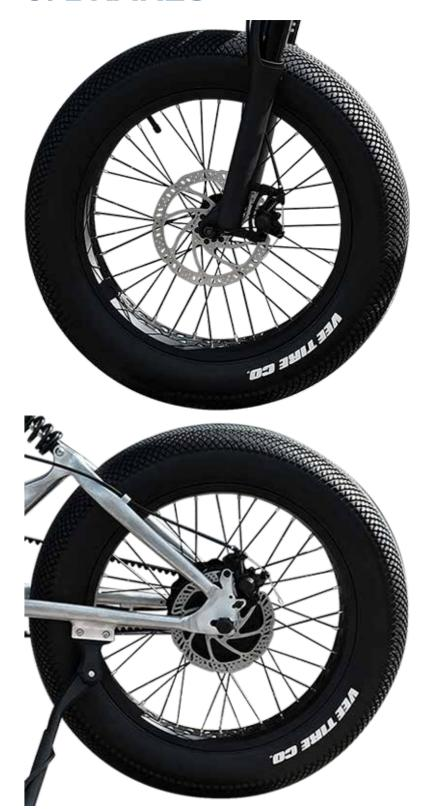
Your Billy ebike comes equipped with front and rear mechanical disc brakes, designed to help you slow down and stop as required.
