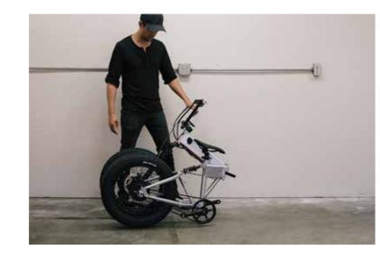
With an anchoring foot behind the rear wheel to stop it from rolling backward as you fold, use one hand to hold the frame close to the seat post and the other hand to hold the front half of the bike. Fold the bike in half using a swinging motion, until the front wheel aligns with the rear wheel. Allow the bike to rest on the lower guard for storage with a smaller footprint.
