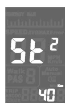
The next setup menu option allows you to set the maximum speed in terms of kilometres per hour. Use the Up and Down buttons to customize your maximum speed.
