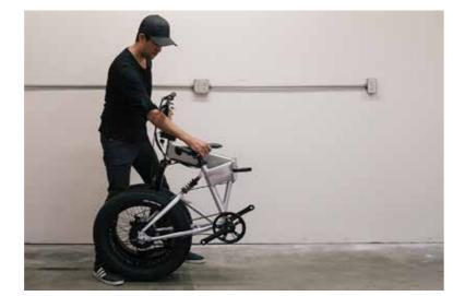
Standing toward the 'tire' side of the folded ebike, place an anchoring foot behind the tire and raise the bike so that the bike is no longer resting on the crank guard.
