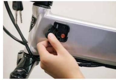
Ensure that the ebike's power button is switched to the off position (0).
