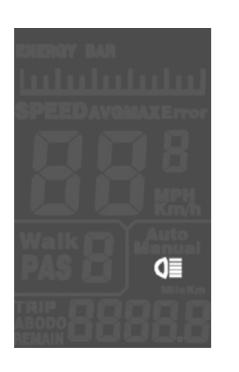
Pressing the Up button for a few seconds illuminates the display for viewing ease when lighting conditions are low. Once illuminated, pressing Up again for a few seconds returns the display to the standard non-illuminated view.
