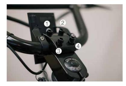
Replace the previously removed top piece and install the four bolts by hand to ensure correct installation.
