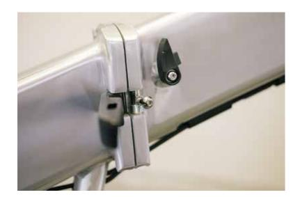
Swing the clamp lever handle outwards to release the clamp.
