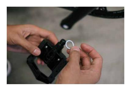
To install the right pedal, find the pedal labelled "R" and place one of the supplied washers on.
