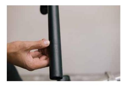
When raising the seat height, ensure that you do not extend the seat height past the minimum insertion point marking on the seat tube.
