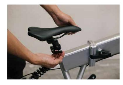
Open by pulling towards the rear of the bike. The seat post should now be loose enough to adjust the seat height.
