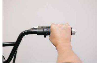
**USA MODELS ONLY:** The right side grip is a motorcycle style twist throttle. Twisting the grip down towards the rider dictates the level of throttle applied.
