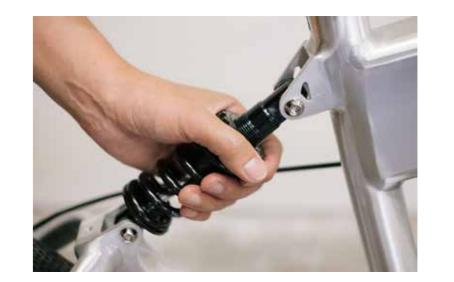
Twisting the stopper in an anti-clockwise direction reduces the amount of preload.
