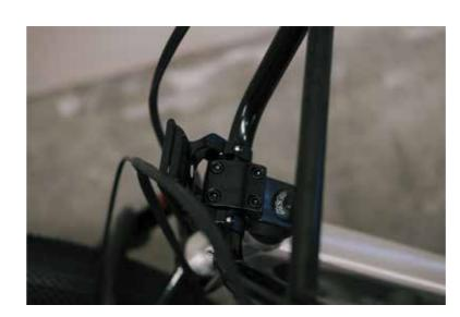
Just before the bolts are fully tightened, adjust the handlebar so that the vertical bars are in line with the forks and the brake levers face forward. Tighten the four bolts to ensure a secure connection of the handlebar to the head stem.
