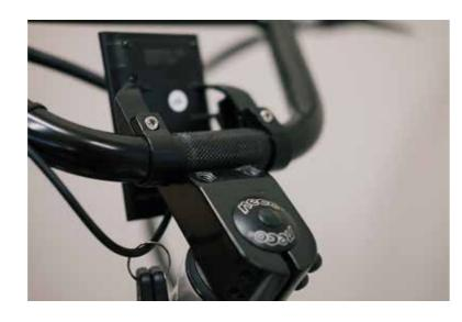
Pointing the handlebars with the levers facing down, place the knurled center section of the bar in mounting point of the head stem.
