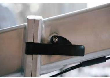
Rotate the lock clasp clockwise so that the locking tab sits inside the hole of the clamp lever handle and the lock clasp sits flush against the handle.
