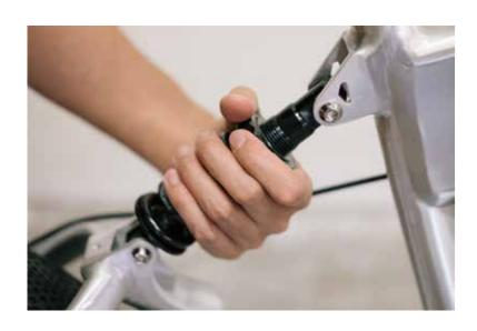
Twisting the stopper in a clockwise direction increases the amount of preload.
