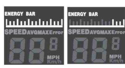
When fully charged, the energy bar across the top right of the display will show bars spanning the width of the display.
