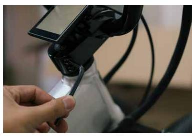
Adjust the display position so that it can be easily viewed when sitting on the bike, then finally secure the handlebar by tightening the two pinch bolts using a 5mm allen wrench.
