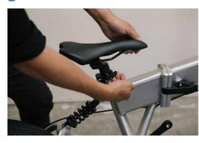
Seat adjustment is achieved without tools via the quick release system. To adjust, locate the quick release lever at the top of the seat tube.
