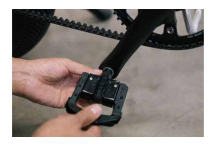
Next, locate the right side crank and attach the pedal to the arm by threading in a clockwise motion.
