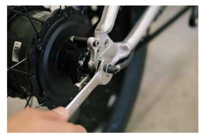
In order to correctly adjust the drive tension, you must first locate and loosen both of the rear axle nuts using an 18mm spanner.
