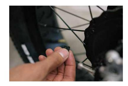
Remove the valve cap by twisting in an anti-clockwise motion.
