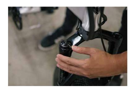
When the dash (-) icon faces closest to the frame, the suspension forks are in full suspension mode.
