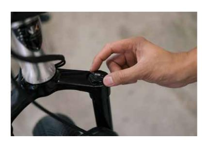
It is also possible to adjust the amount of preload on the air suspension.
