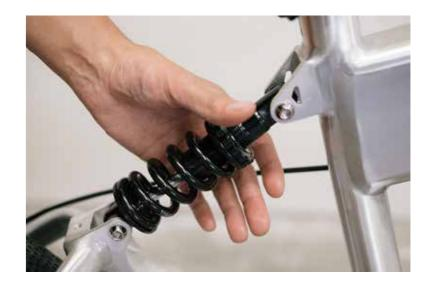
To adjust, locate the textured threaded stopper that sits at the end of the suspension spring, towards the top of the rear suspension unit.
