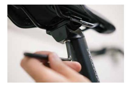
To adjust, loosen the securing bolt with a 5mm allen wrench and turn in an anti-clockwise direction.
