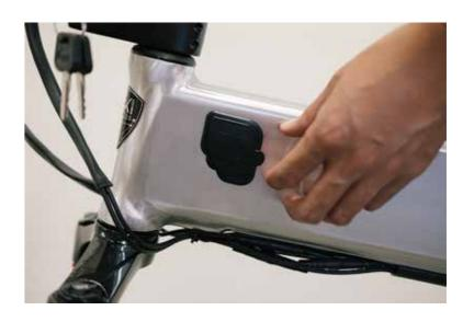
Your battery can be charged either on or off the ebike. To charge on the ebike, locate and peel open the rubber door to expose the battery's ports and power button.
