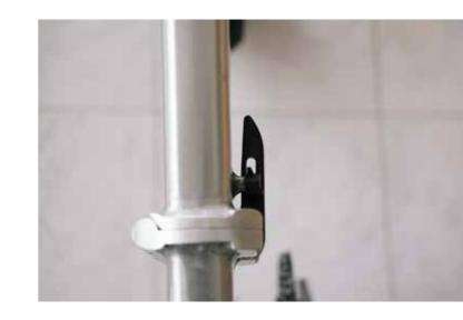
Clasping the clamp lever handle, draw it closed by swinging it across the frame break so that there is an even gap between the lever handle and the front half of the frame. It is designed to sit very close to the frame, but not actually touch it.
