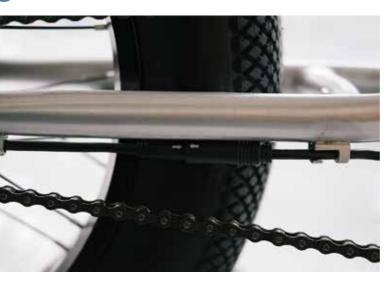
Ensure the motor cable is securely connected to the controller connector cable.
