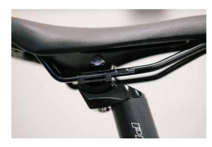
Once the bolt is loose enough, there should be enough play in the seat rail clamp to allow the seat to slide back and forth. Ensure that you only slide the seat so that the seat rail clamp's edges sit within the range marked on the seat post rails.
