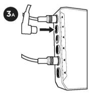
Insert the foot motor cable (has red band) into the slot labeled foot motor on the control box.
