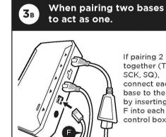
If pairing 2 bases together (TXL, SCK, SQ), connect each base to the other by inserting part F into each control box.
