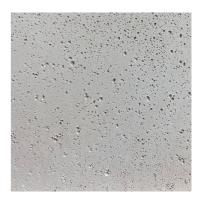
Pinholes are where air bubbles occur in the concrete during the casting process. They will vary in size and number with each product cast and are very much a part of concrete's distinctive feature.
