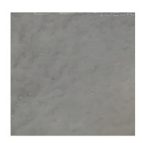
Flow lines occur when concrete, in it's liquid state, is poured into a mould. They are often more prevalent in straight-sided or tall products.
