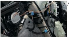
Now mount the Diamond Audio speaker by pushing it in and connect it to the factory cable of your vehicle. Mount the door trim in reverse order.
