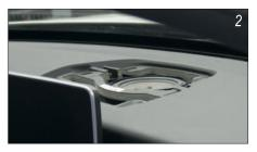
Lever out the speaker grille. Then loosen the old speaker (lever out, not screwed).
