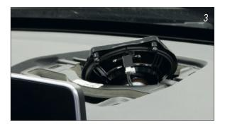
Remove existing plugs from the loudspeaker.
