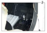
Remove the door strip and the cover under the glove If present, remove the plug from the cover.
