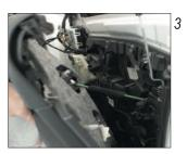
Remove the two screws on the door handle (TX27) and carefully lever the door trim out (from bottom to top). Now remove all the plugs that are connected to the door trim.
