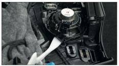
The speaker is now accessible. The speaker is not screwed on. Lever out the speaker and remove it.
