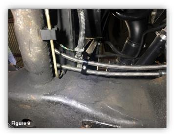
The return line will pass directly up, in front of the core support, and will connect to the passenger side of the transmission cooler (SEE FIGURE 10). The pressure line assembly will follow the underside of the core support towards the driver side (SEE FIGURE 11) where it will then pass up in front of the core support and connect to the driver side of the transmission cooler (SEE FIGURE 12).
