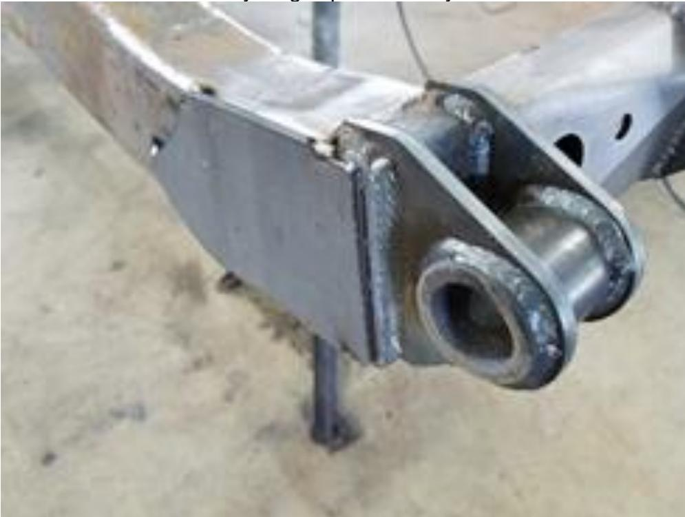
With the plates tacked in place you can now see how the ends will be fully closed off. Once you have confirmed all the pieces are aligned properly you can weld the cross member and side plates to the frame.
