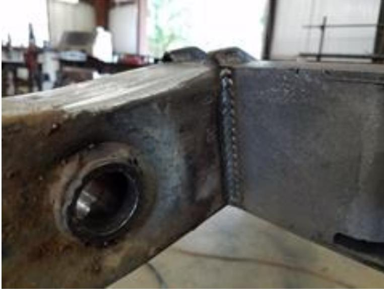
Once all pieces are fully welded and cooled down you can install bushings, shackles, leaf springs and the rest of the components.
