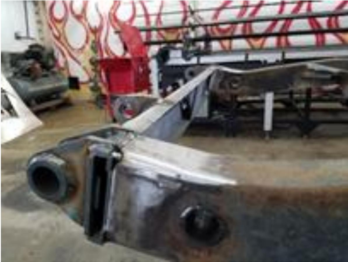
The frame rails will end up even or flush with the end of the cross member like shown. An end plate will be welded to close this off. Next, place the new cross member against the frame rails to ensure it is square and centered. Tack weld into place. The frame side plates can now be added to cap off the end of the cross members and tacked into place.
