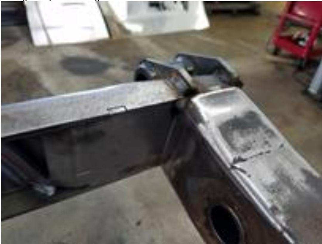
Make sure the cross member sits flush with the frame rails so that you can get a good weld onto the frame.
