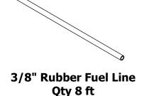
Connect 3/8" Fuel Line to Barbed Splice. Install 3/8" Hose Clamp. Route 3/8" fuel line from EVAP hose to inner fender. Add a loop in the hose. This will provide an air loop for the rollover valve, allow expansion of fuel vapors & prevent fuel entering the EVAP canister. Connect 3/8" fuel line to Rollover valve on tank. Install 3/8" Hose Clamp.
