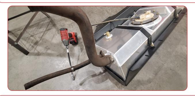
Raise the tank back into the jeep in the factory location and reattach the fuel lines, fuel filler hose to the filler neck assembly, wiring harness, EVAP lines, and vent line. The EVAP lines, if equipped will need to be adapted to fit. The -8AN fitting can be used as a return line, adapted to the EVAP system, or blocked off completely.
