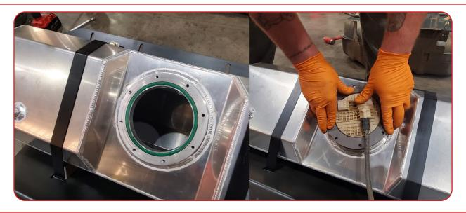
**11**) Install the roll over valve / vent in the top of the tank.
