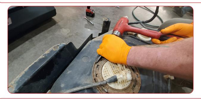
Remove the pump from the factory tank and remove the O-ring to be reused on the Motobilt aluminum tank.
