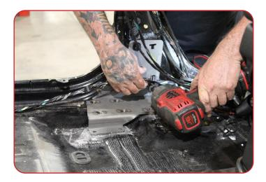
Mark the three holes that need to be drilled. Drill the three holes that bolt MB3032-06 to the tub floor to allow a 3/8" bolt to pass through.
